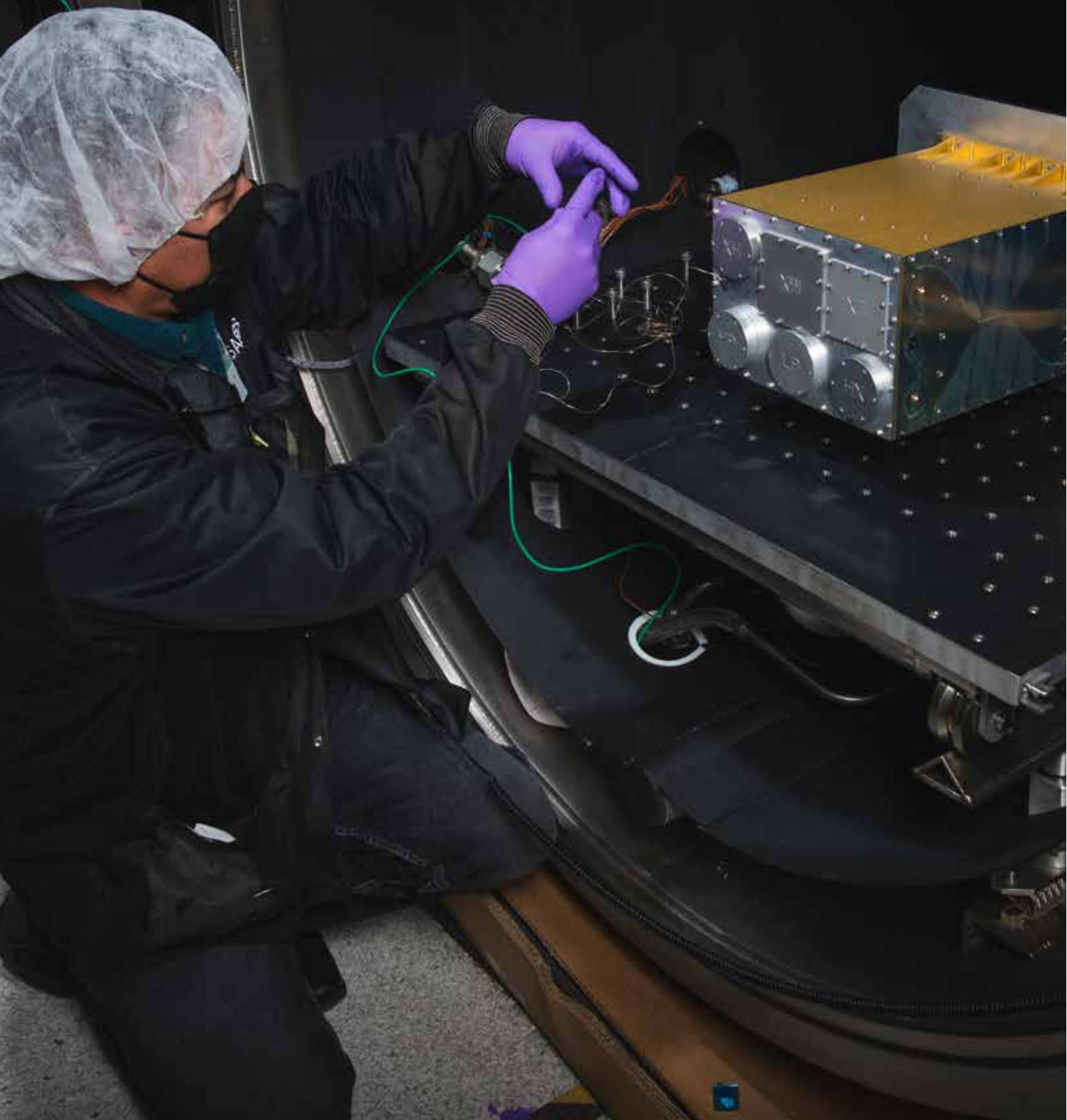
■ Vernon Vigil, Space Instrument Realization group thermal/vacuum test lead, applies temperature monitors to a HRS test unit. The HRS will be used on 22 future GPS satellites scheduled to launch starting in 2026.
